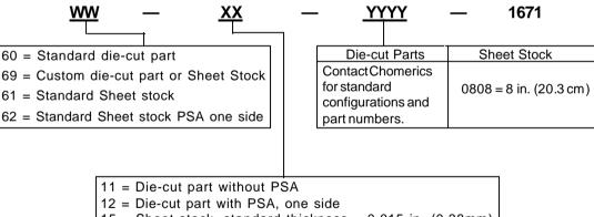
15 = Sheet stock, standard thickness = 0.015 in. (0.38mm) Contact Chomerics for custom thickness part numbers
