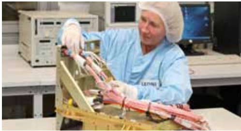
Cable harness production and installation into an Ariane V5 TMO-Container by LEONI.
